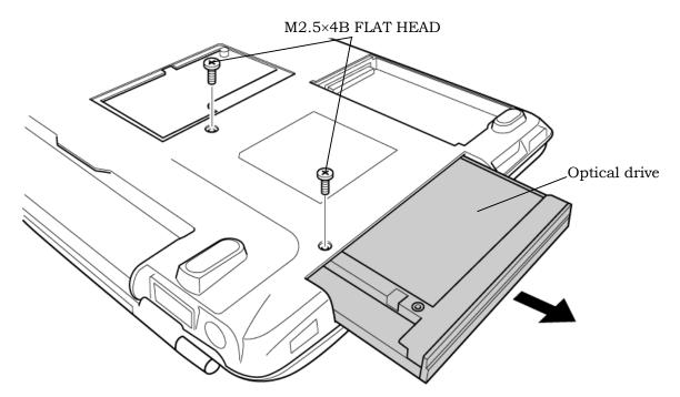
Figure 4-6 Removing the optical drive
